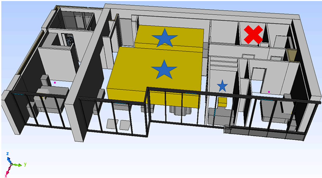
Fig. 9. Location of the three occupants (three blue stars: two adults in the kitchen/living area and one child in the office area) and places with a good likelihood of CO 2 generation (yellow volumes). (For interpretation of the references to colour in this figure legend, the reader is referred to the web version of this article).
