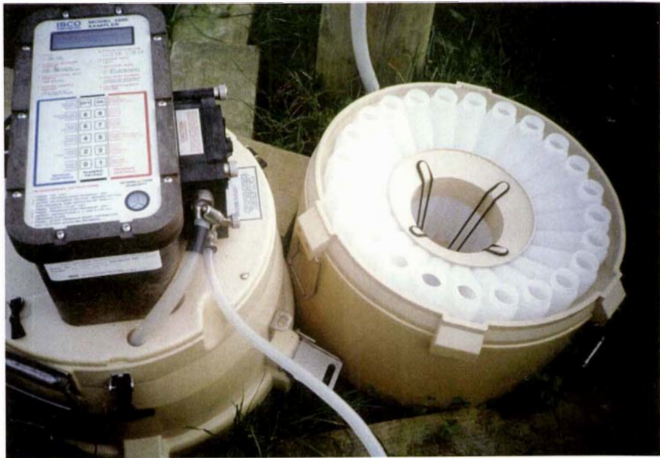
. 2.5 The automatic water sampler used for collecting drainage samples for analysis
