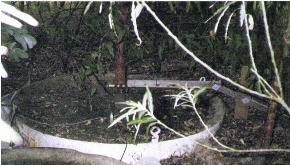
Figure 2.1 An E. saligna lysimeter showing the irrigation sprinklers. The lysimeters were 1.0 m deep and 1.8 m in diameter.
