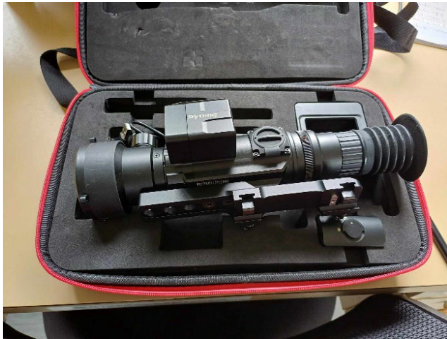
Figure 2.4 The thermal imaging scope used in this study. Sytong RM03-35LRF.
