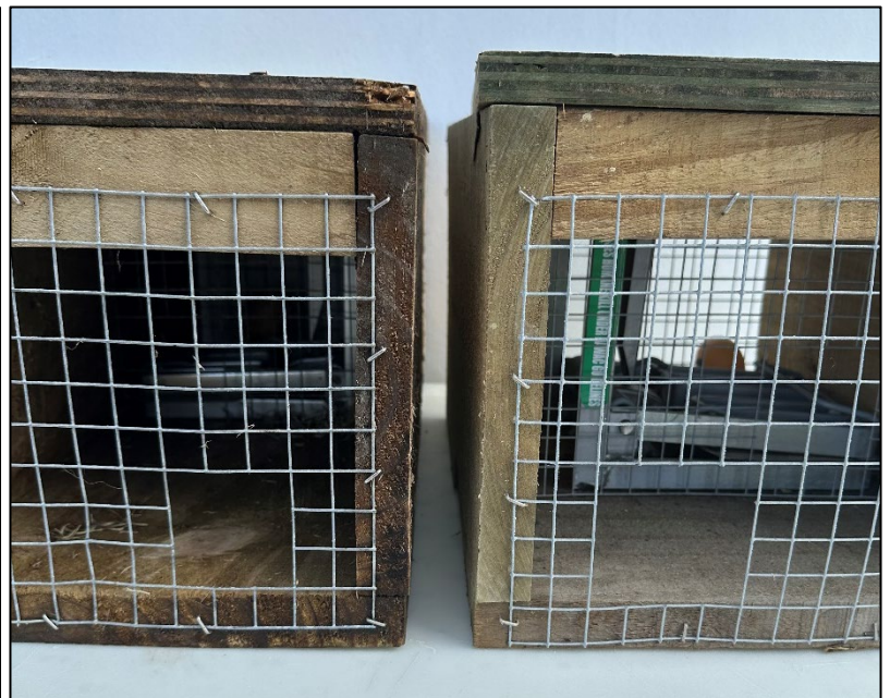
Figure 6.2 Front-on view of the standard baffle aperture size for a DOC200 (left; 60 mm by 60 mm) versus a DOC250 (right; 80 mm by 80mm).
