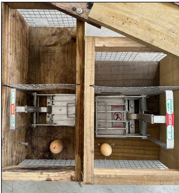
Figure 6.1 A DOC200 trap (left) versus a DOC250 (right) trap. Note: the DOC200 is a “weka-proof” style with a longer distance between the first and second baffles.
