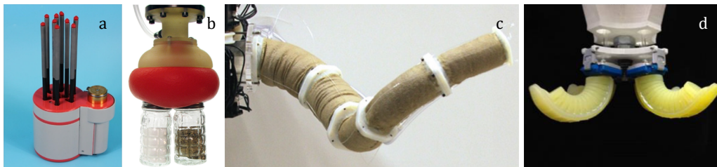
Figure 2.13. (a)—meshed pin-array structured end-effector [282, 284]. (b)—universal gripper based on granular jamming [286]. (c)—highly articulate tubular gripper design [291]. (d)—soft pneumatic robotic gripper design [293].
