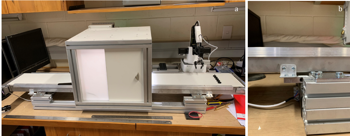
Figure 9.5. Illustration of the conveyor system. (a)—front view of the constructed prototype. (b)—10 kg load-cell used to find the COG of an object.
