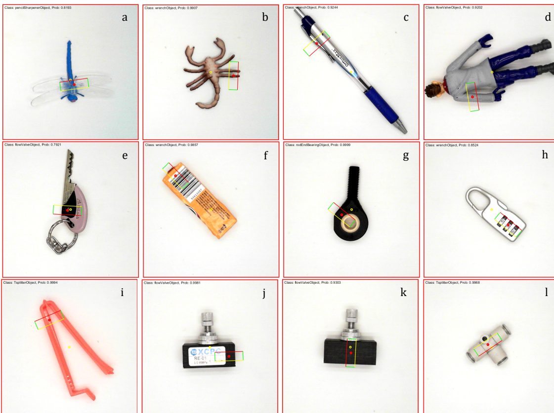
Figure 10.28. Various selected grasps resulting in a fail label and generally very poor OS and OE scores. (a)—blue dragonfly toy (uH011). (b)—brown scorpion toy (uH007). (c)—blue Officemax pen (mT005). (d)—fixed figurine (mH004). (e)—key (uH006). (f)—PK chewing gum (mH010). (g)—rod end bearing (kC002). (h)—silver combination lock (uT015). (i)—red sealer (mH009). (j)—XPC pneumatic valve - no fittings (mC008). (k)— XPC pneumatic valve - no fittings (mC008). (l)—pneumatic T-splitter (kC004).
