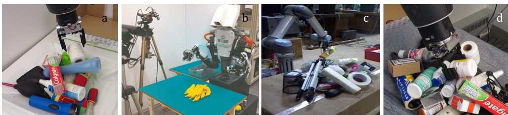
Figure 2.24. (a)—example of cluttered grasping from an unstructured pile using point cloud grasp pose detection [41]. (b)—picking a cylindrical object from an unstructured pile [56]. (c)—picking a specific object from a heap of objects [330]. (d)—example of novel object grasping in dense clutter [62].
