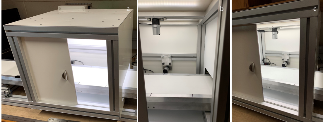
Figure 9.9. Various images related to the vision enclosure of the constructed prototype. (a)—frontal view of the complete enclosure. (b)—internal view showing relative camera placement. (c)—internal view showing cameras and beam sensor.
