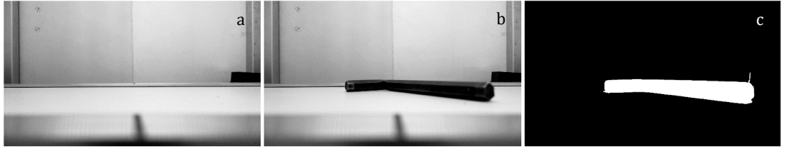
Figure 4.20. Example of the side-view segmentation process. (a)—reference image I_{s_{blank}} captured prior to object introduction. (b)—side-view image I_s captured post object introduction. (c)—thresholded difference image I_{s_{Th}} .
