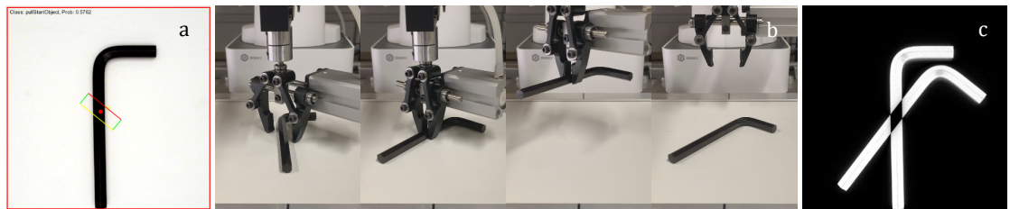
Figure 3.7. Example of rotational error. (a)—grasp selected for implementation. (b)—sequence of images illustrating the grasp trial. (c)—resultant difference image between pre-grasp image and post-grasp image.
