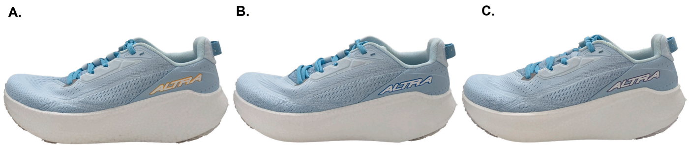
Figure 1. Photographic representation of the three test shoes, which differ only in midsole density ( \rho ), where (A) = 0.164, (B) = 0.147, and (C) = 0.122.
