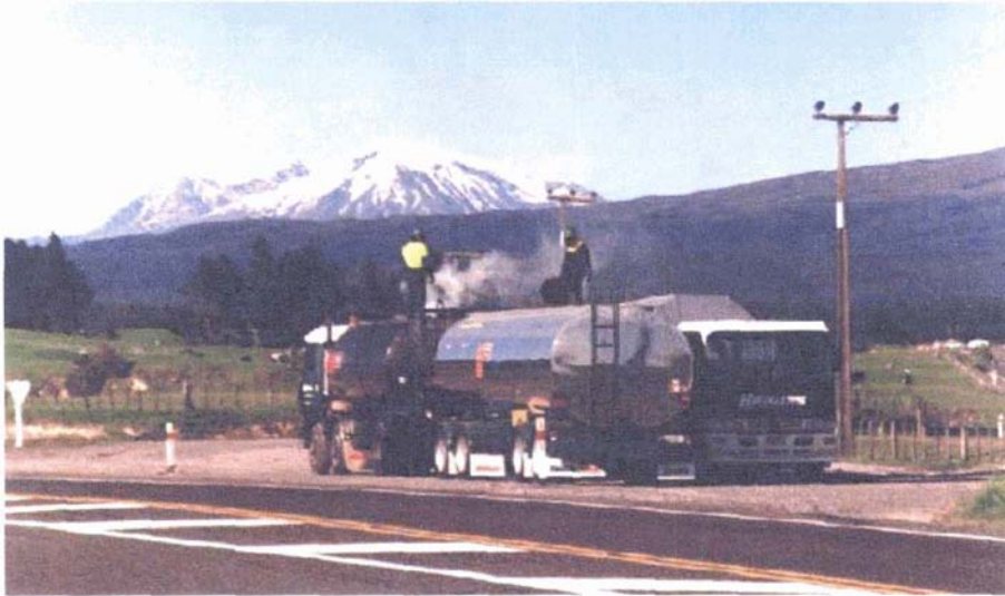
Figure 3.1: These bitumen carriers are transferring part of the load from one vehicle to a second. The first vehicle has travelled from the company's base in the east of the North Island of New Zealand to this siding at an intersection in the Central North Island. Having completed the transfer, the two vehicles will carry on to complete road maintenance in two different areas. The site chosen for the transfer is a layby at an intersection.
