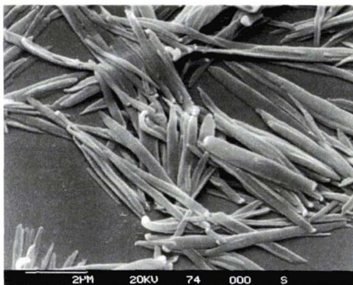
**Figure 5.35 Growth CV (top) and SEM image of XXVI film on ITO-coated mylar**
