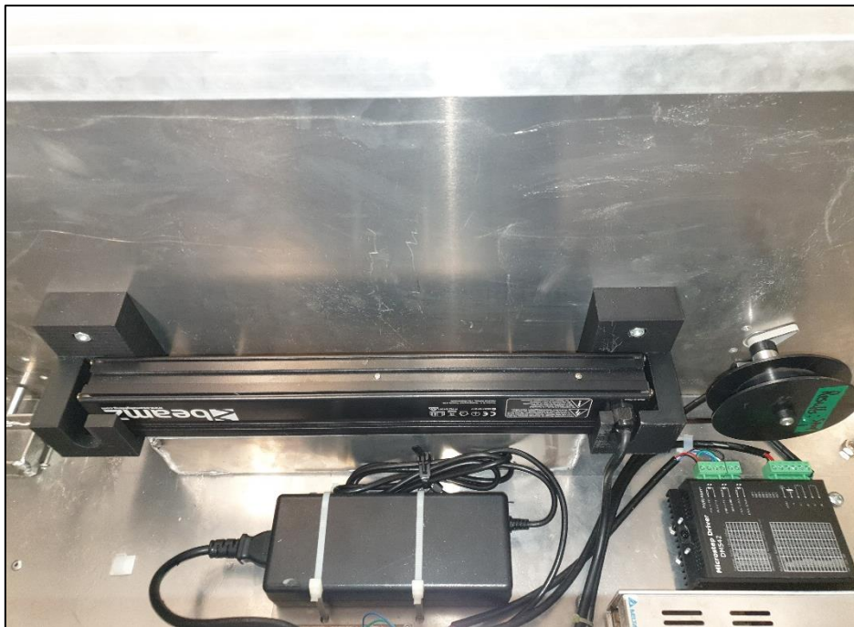
Figure 4-49 - The Carbon Fibre Yarn passing underneath the UV Light and onto the Secondary Spool.
