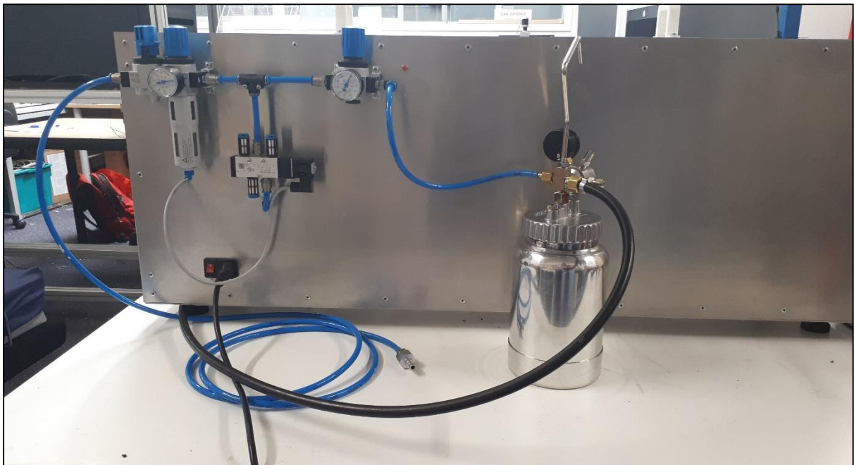
Figure 4-44 - The Pneumatic Circuit Mounted onto the Frame for Prototype 3.
