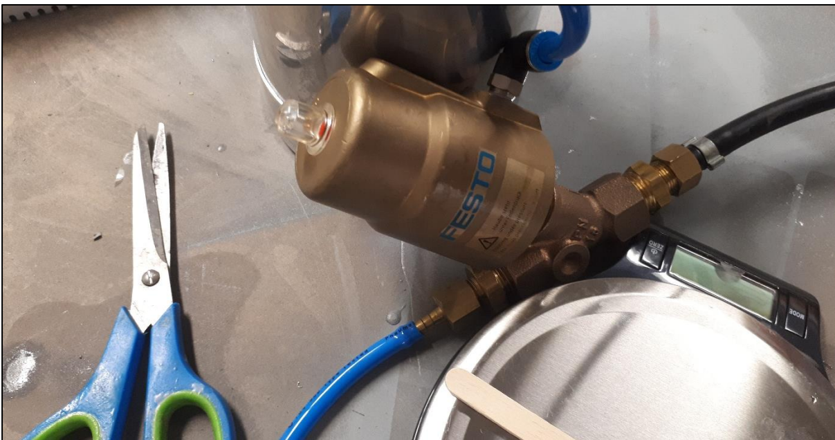
Figure 4-43 - The Angle Seat Valve used in Prototype 3.
