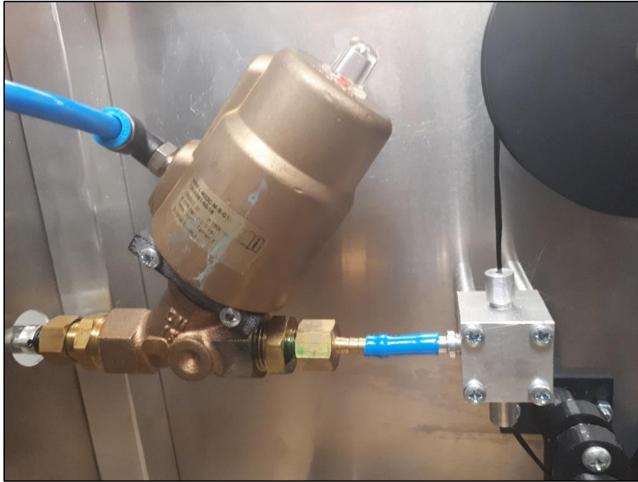
Figure 4-45 - The Angle Seat Valve mounted in Prototype 3.
