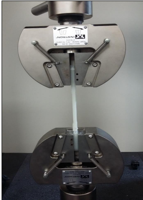
Figure 5-6 - Type I Specimen inside an Instron using the 2716-015 Wedge Action Grips.
