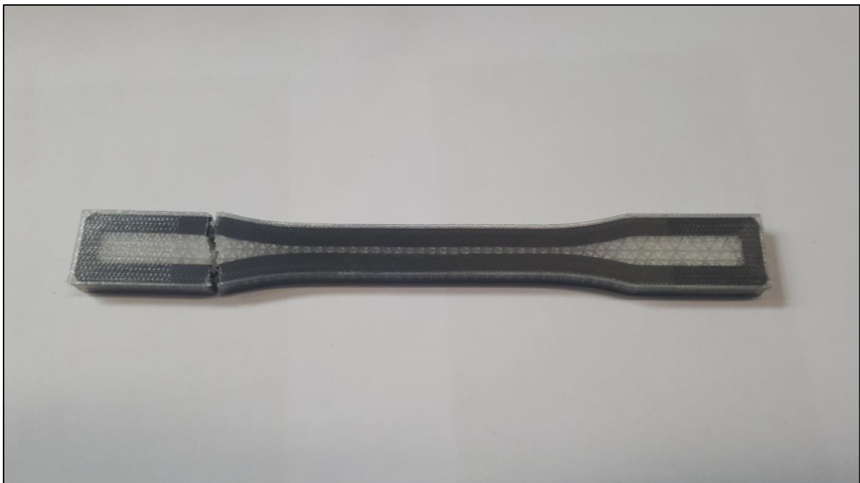
Figure 5-11 - Type I Specimen that has Fractured prematurely during Tensile Testing.
