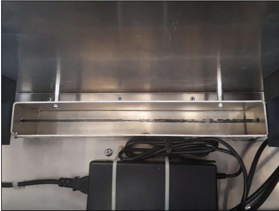
Figure 4-48 - The Carbon Fibre Yarn passing through the Aluminium Tray.
