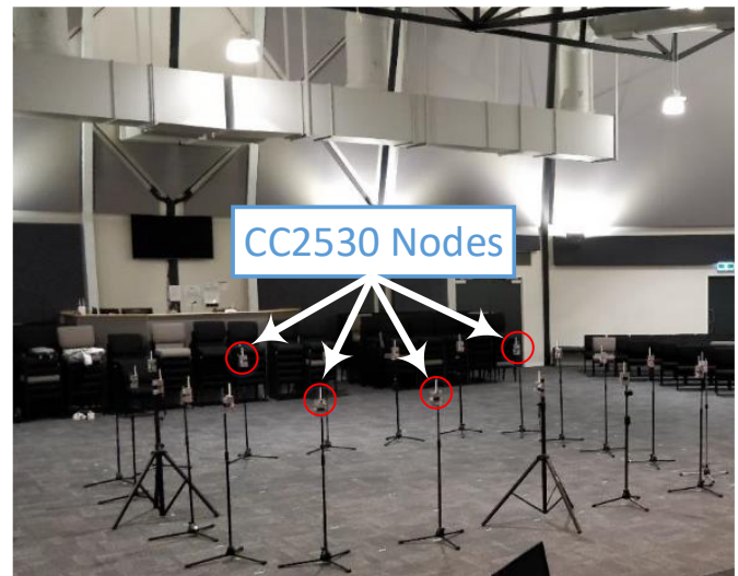
Fig. 5. Auditorium Node Placement
