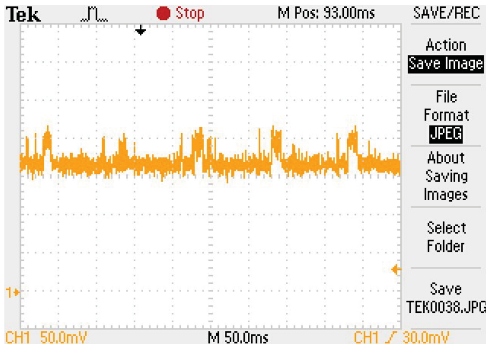
Figure 77: The Voltage Signal when Always Awake
