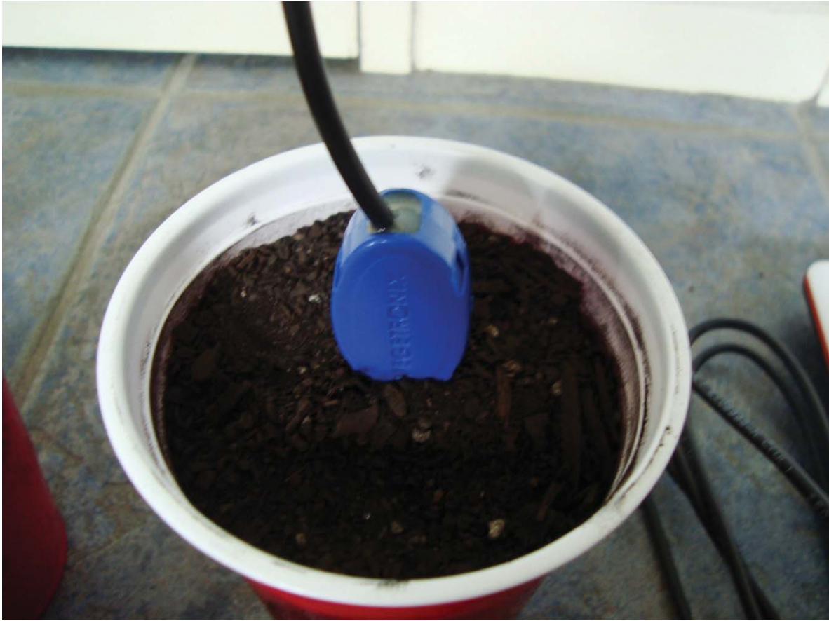
Figure 18: VG400-LV Sensor Inserted into Soil for Soil Moisture Measurement
