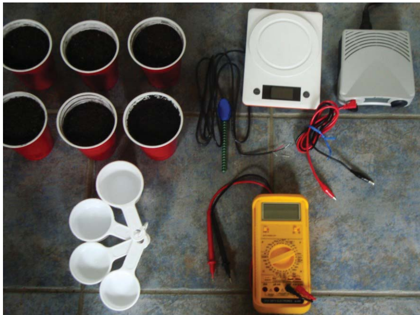
Figure 17: Tools used for Obtaining Relationship of Voltage Output for VWC in Potting Mix for VG400-LV Sensor
