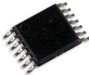
Figure 33: The Surface Mount Device AD8302 Gain Phase Detector [38]
