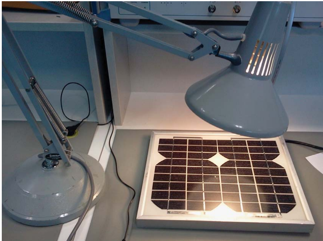
Figure 85: Testing Procedure with Solar Panel and Lamp as Light Source
