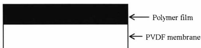
Fig. 6.7. Schematic of a bender made by casting polymer as a solution in chloroform on a PVDF membrane strip.
