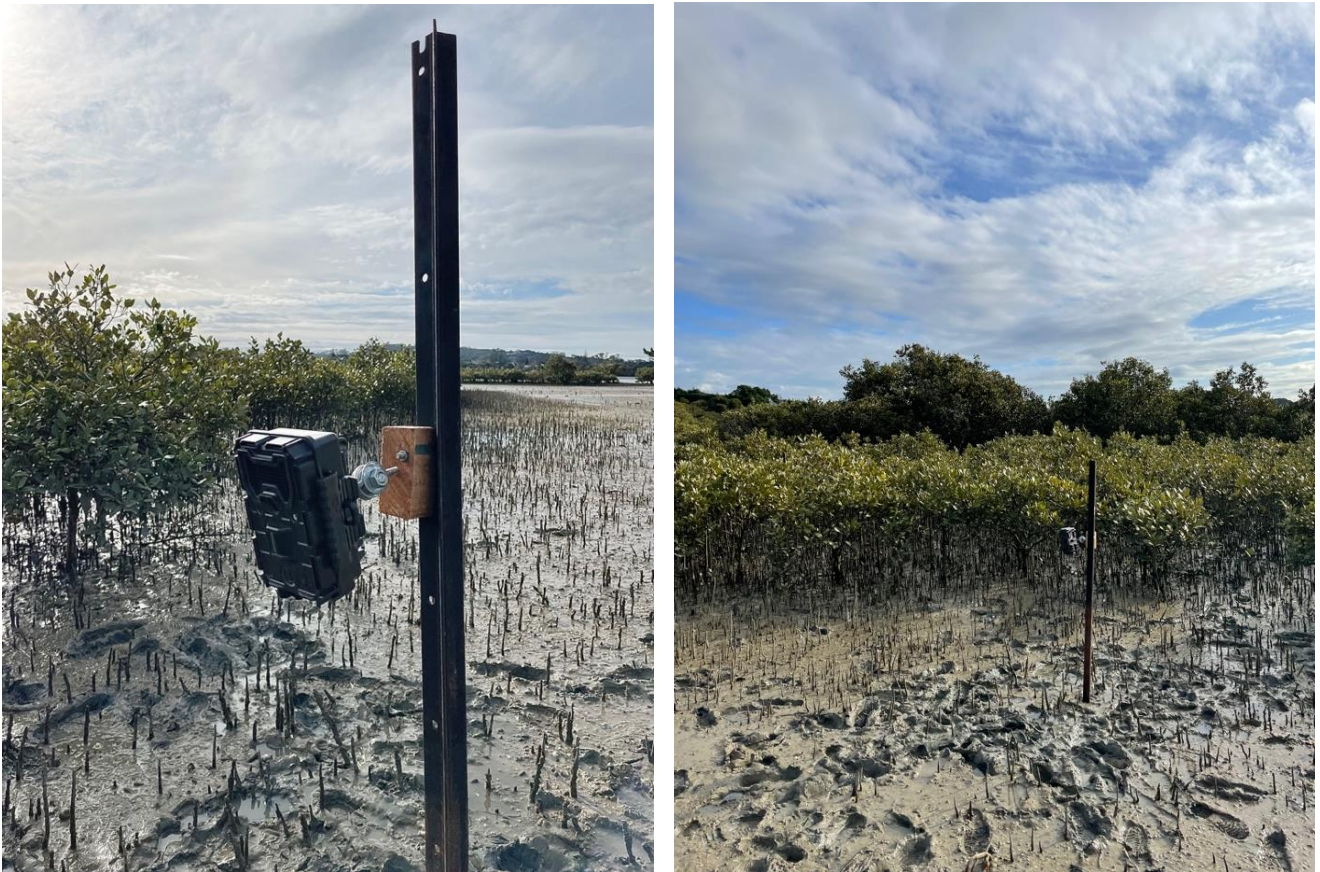
Figure 3.5: Photographs showing a camera trap securely mounted on a metal post using a wooden mounting piece and bolt (Left), and the camera traps' positioning in the field (Right) at Summerset Village in the upper Waitematā Harbour, June 2022. Photographs by I. Mallinder-Capamagian.
