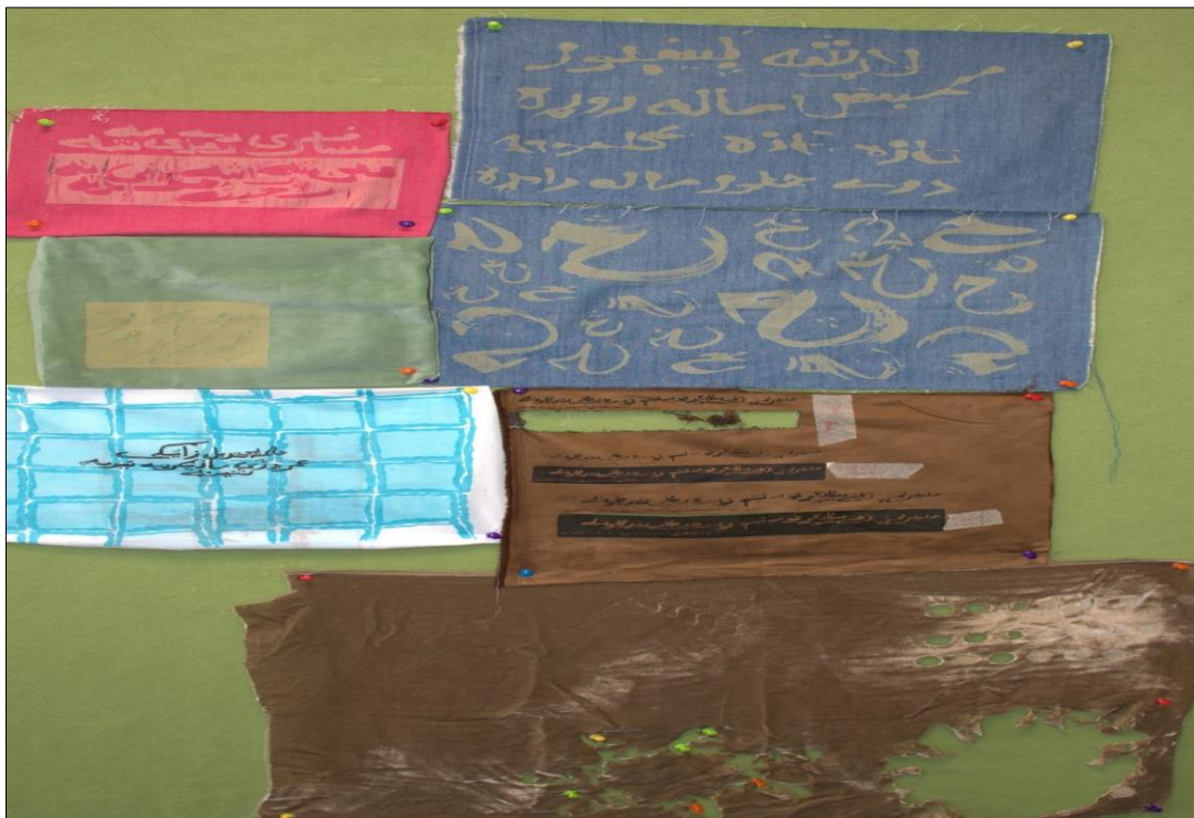
Figure 4.6: Fabric samples including denim, suede, velvet, and upholstery velvet tested for digital embroidery and laser etching. Velvet proved the most aesthetically pleasing but presented significant technical challenges. Photograph by the author, November 2024
