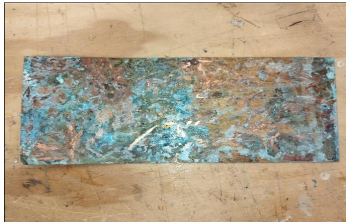
Figure 4.37: Copper sheet treated for patina effect, prepared for punching into coins. May 2025
