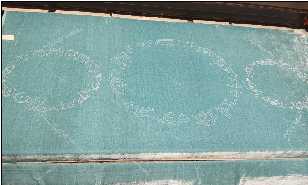
Figure 4.41: Rasterized velvet fabric. Shawl placed on the laser bed. June 2025
