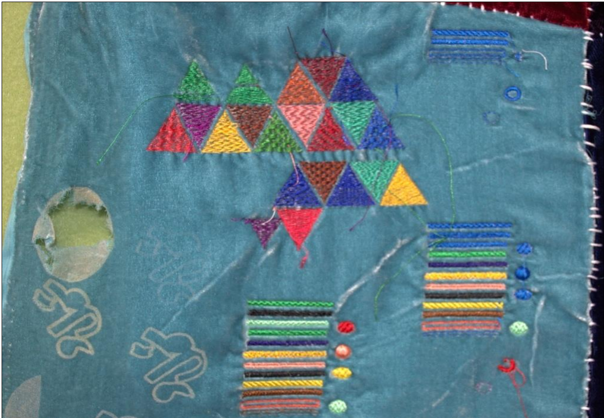
Figure 4.8: Different laser power percentages and speeds tested on velvet fabric using rasterizing technique, showing varied outcomes in laser etching and embroidery quality. Photograph by the author, February 2025.
