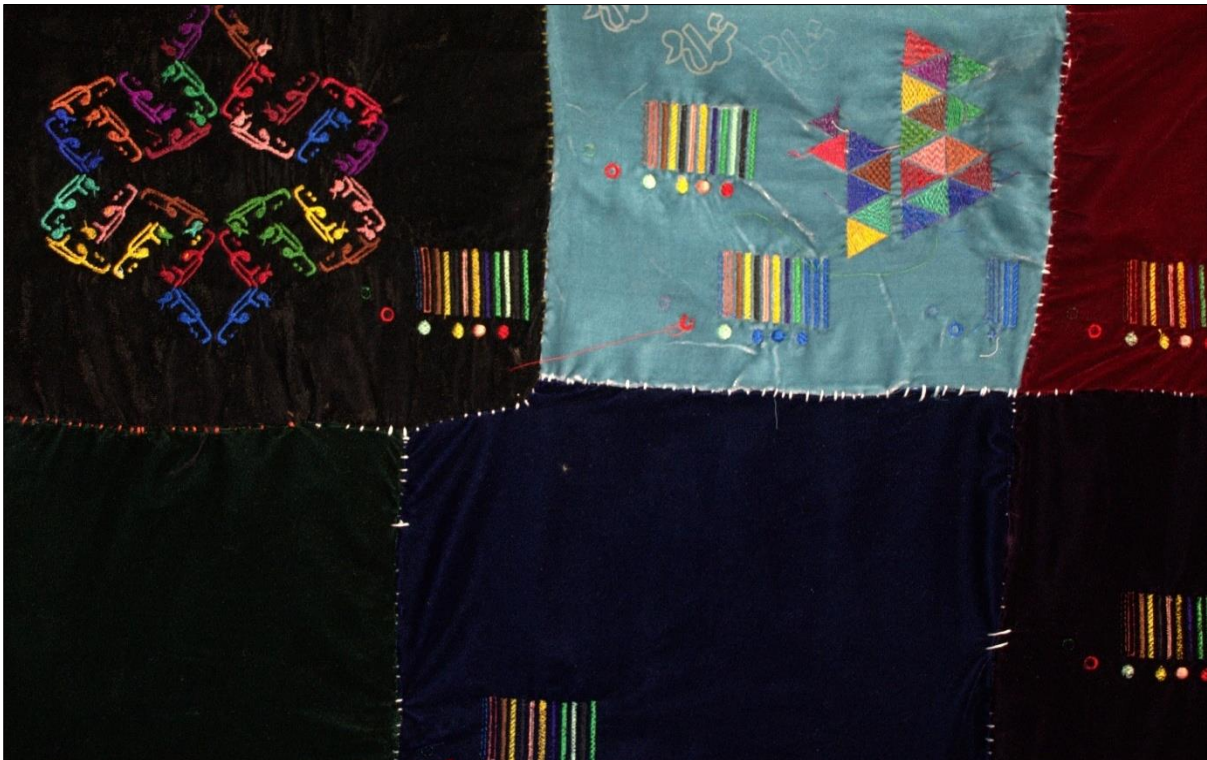
Figure 4.7: Various fabric samples tested: suitable for embroidery but unsuitable for laser etching except the turquoise one. Photograph by the author, February 2025.
