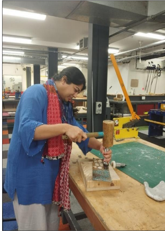
Figure 4.38: Punching the copper sheet at the 3D workshop. May 2025.
