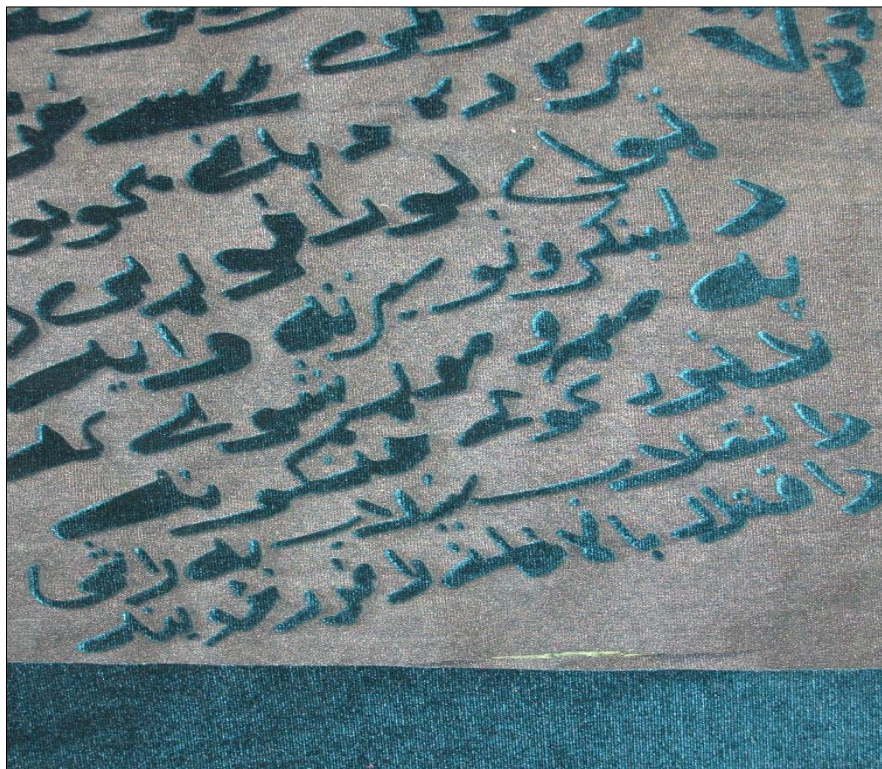
Figure 4.4: Sample of velvet that frayed and began to rip after a few days, highlighting the material's unsuitability for long-term use. Photograph by the author, May 2024.
