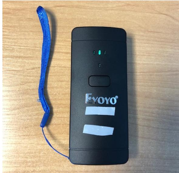
**Figure 3.11 Pocket 2-dimensional (2D) barcode scanner.**
