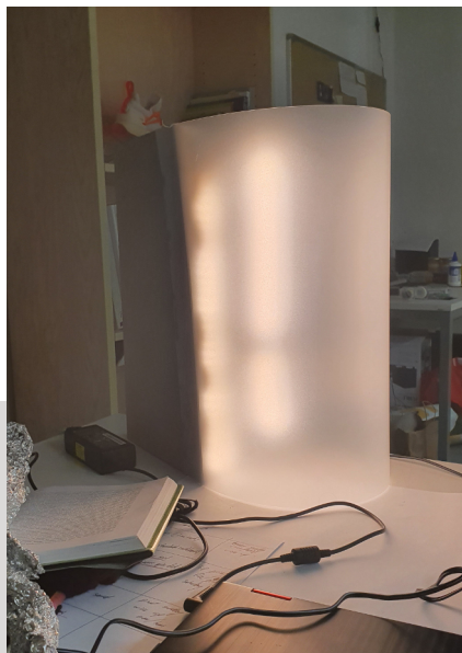
Figure 15 The Shadow lamp. Uses two strips of LED's to project a shadow on to the screen as seen in figures 11-13.
