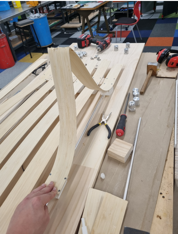
Figure 66 Testing the flexibility of the bamboo
