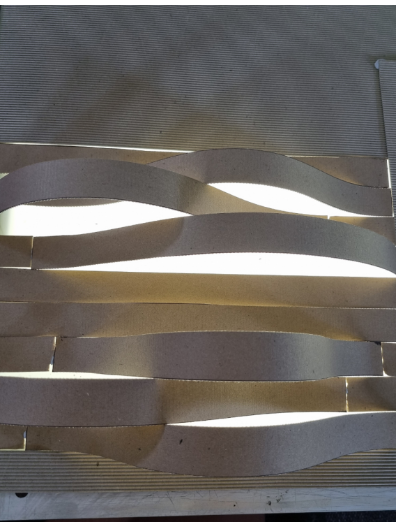
Figure 58 How the lights look with light. As the slats bend and contract more light is able to fill a space
