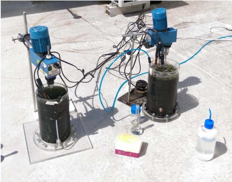
Figure 2 - 3: Bench experiment full set up during light assay. Gas bubbling is visible in the reactor on the right
