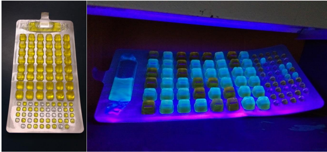
Figure S5 - 1: Quanti-tray results example: readings under normal light for total coliforms counting (left) and fluorescence under UV-light for E. coli counting (right)
