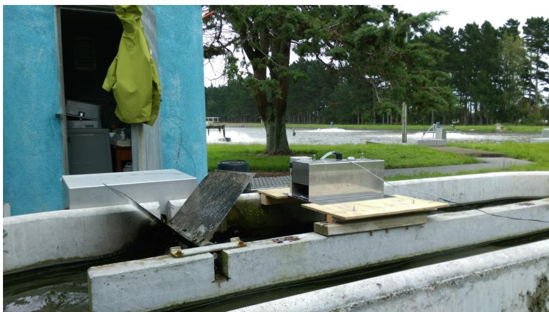
Figure S3 - 1: Tipping bucket set up at the inlet of HRAP A for accurate wastewater flow rate monitoring
