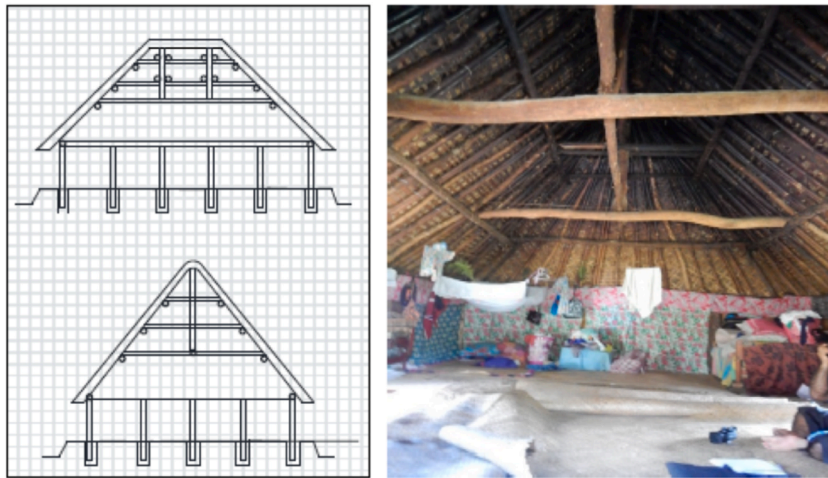
Fig. 11. Structure of a bure without a centre post (left); crossbeams and posts holding the ridge beam (right) (Source: Author).
