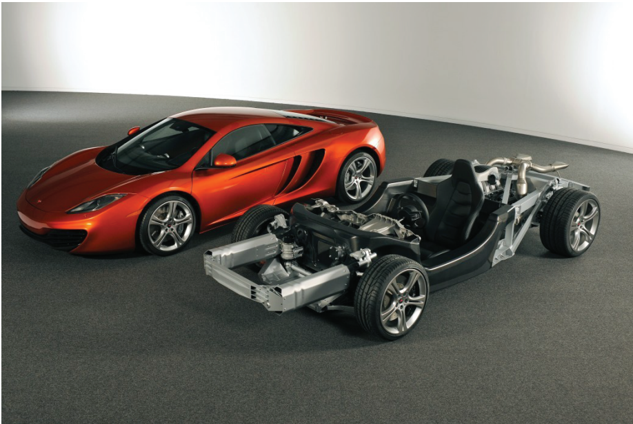
Figure046 "Semi Monocoque - McLaren MP12-C"
