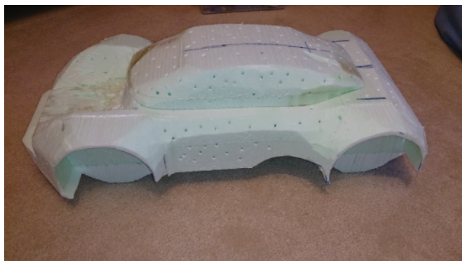
Figure080 "Clay Model Process Images"
