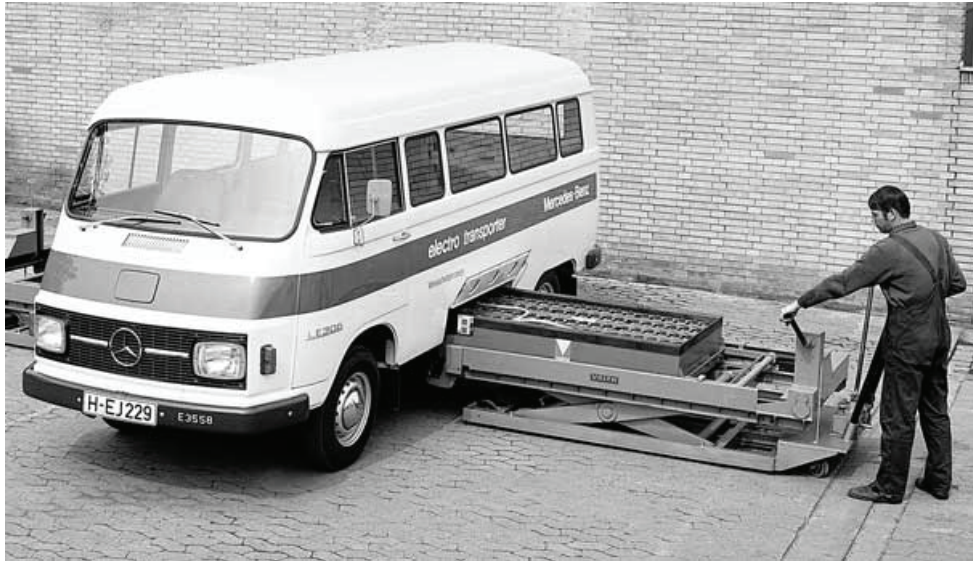
Figure039 “Mercedes N1000 Electric Test Model , Battery Change 1972”
