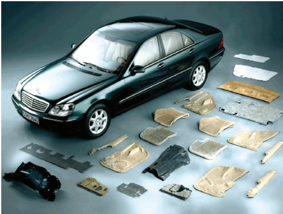
Figure033 "Mercedes S-Class W220 Use of Natural Fibres"
