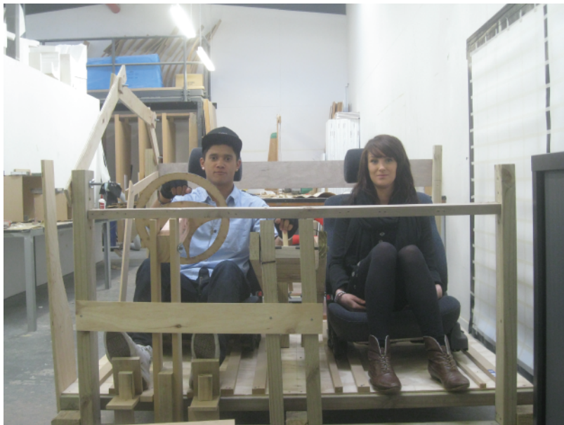
Figure060 "Interior Box - Ergonomic Tests Images"
