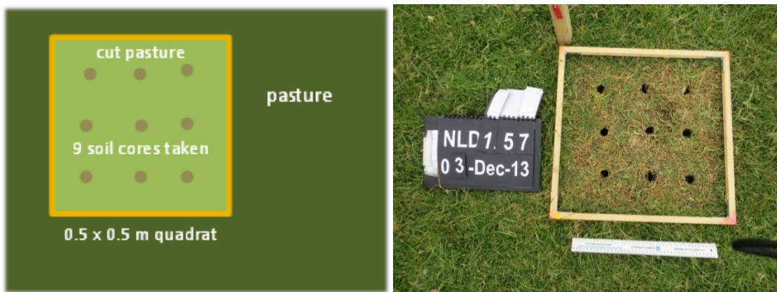
Figure 3-34: Diagrammatic representation of the soil cores collected within the sample quadrat and photograph of a plot after soil coring.
