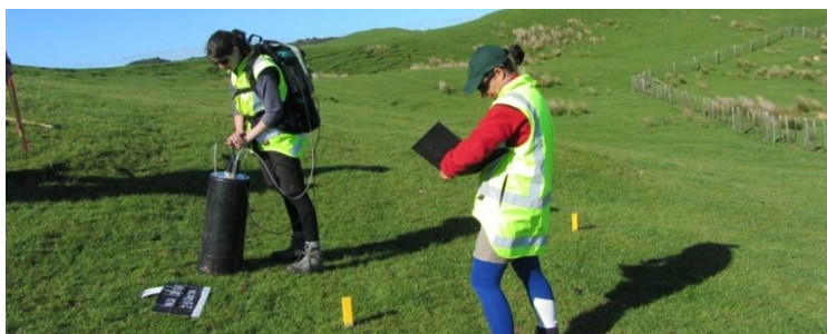
Figure 3-32 Measuring pasture canopy reflectance in the field at Limestone Downs.
