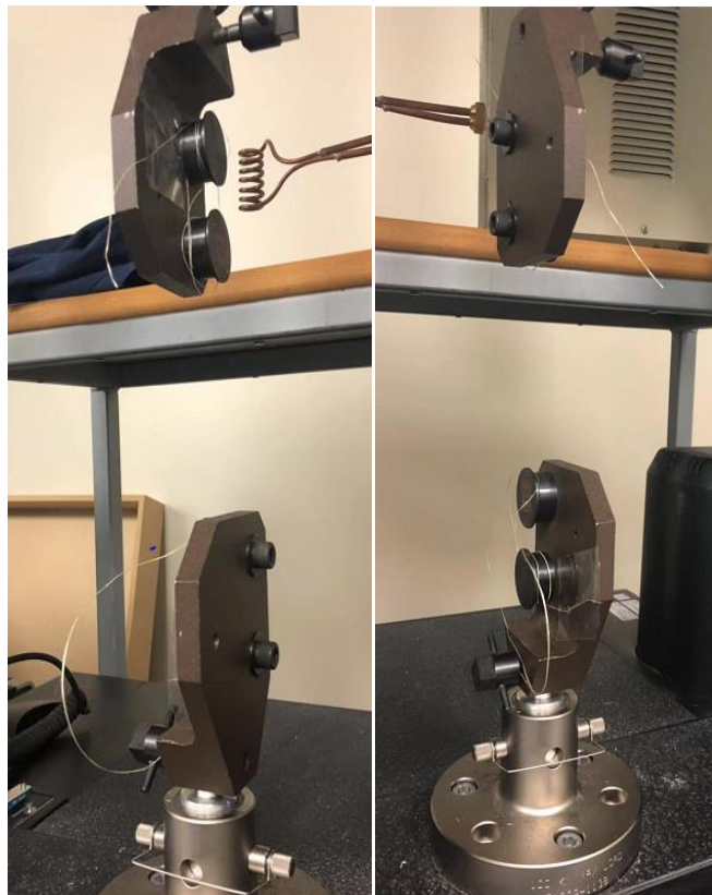
Figure 65 Tensile test of Harakeke Fibre with clean break
