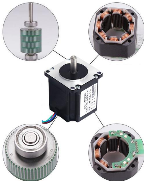
Figure 17 Internal structure of stepper motors
