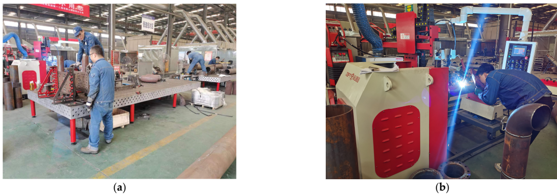
Figure 7. Semi-automatic processing schematic diagram of the preform factory. (a) Pipe docking on the pipe prefabrication platform; (b) semi-automatic welding.
