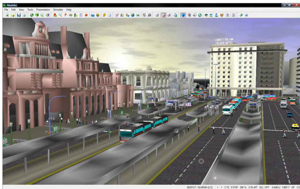
Figure 2.3: Paramics Modeller traffic simulation running, showing three dimensional representation using the available graphics libraries to preview buildings around the traffic network, as well as traffic members such as cars, trucks, public transport and pedestrians [36]
