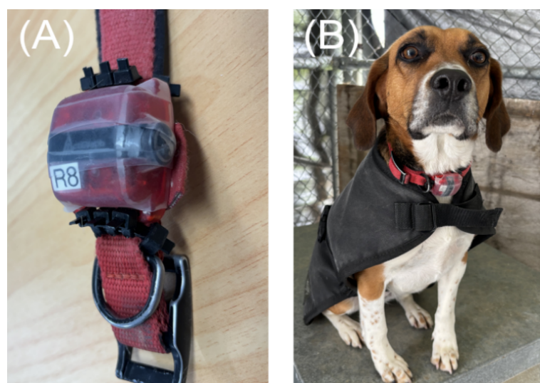
Figure 2.5 Accelerometer placement and coat fitting showing (A) Close-up view of the accelerometer wrapped in waterproof tape and fixed to a collar (B) a dog fitted with a coat and accelerometer secured to the collar.
