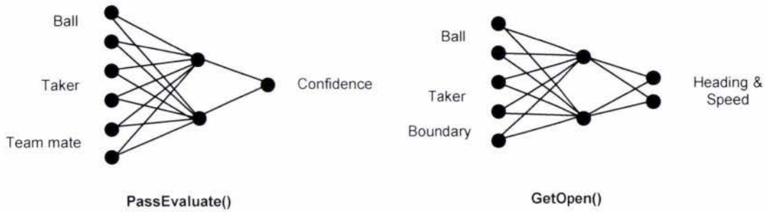
Figure 3.2: Example network topologies for the PassEvaluate() and GetOpen() functions.
