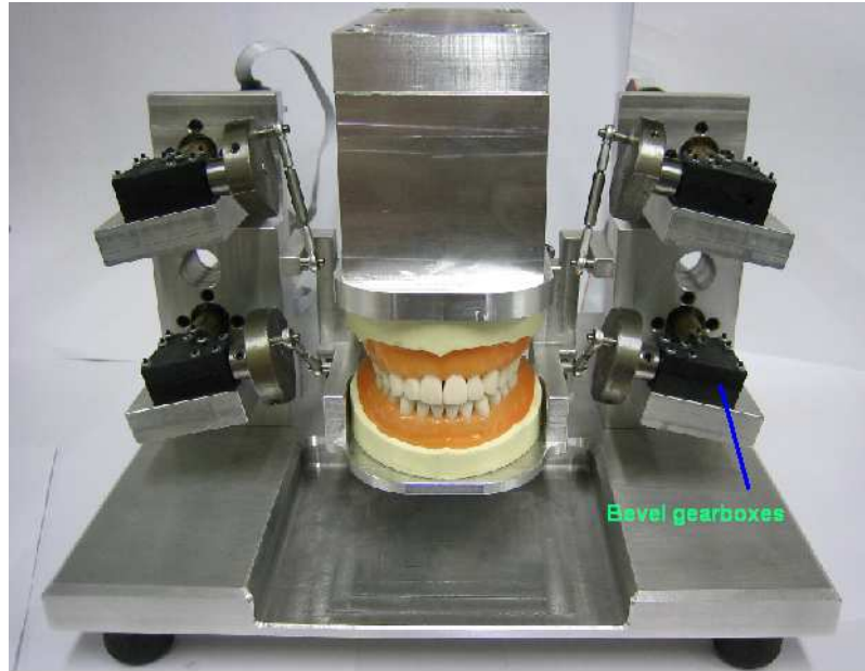
Figure 3.1 Built masticatory robot
