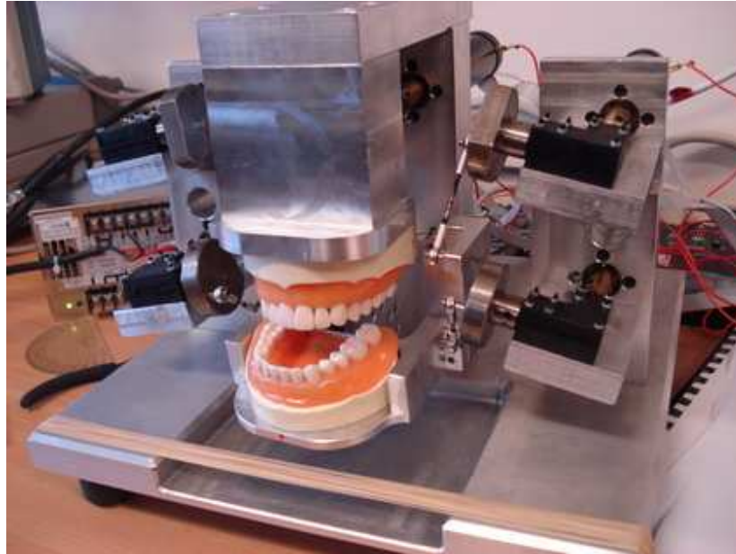
Appendix Figure 2.1 Massey robotic jaw running free
