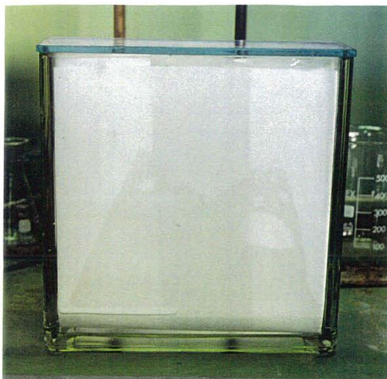
Figure 3.3 Glass tank-blotter paper system used for separation of substances in cucumber leaf extracts spotted on thin-layer chromatograms
