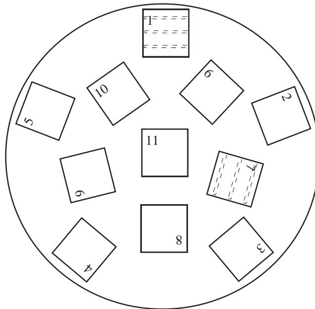
**Figure 4.3** Position and numbering of glass cover slips placed on Corflute disc for evaluating ascospore distribution within the Burkard settling chamber. Dashed lines on cover slip 1 and 7 indicate the relative orientation of three transects on each cover slip.
