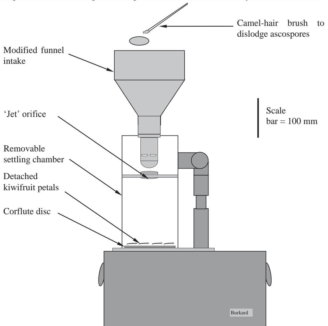
**Figure 4.1** Burkard high throughput 'Jet' sampler with modified intake used for inoculation of detached kiwifruit petals with dry *S. sclerotiorum* ascospores, referred to as the 'Burkard settling chamber'.
