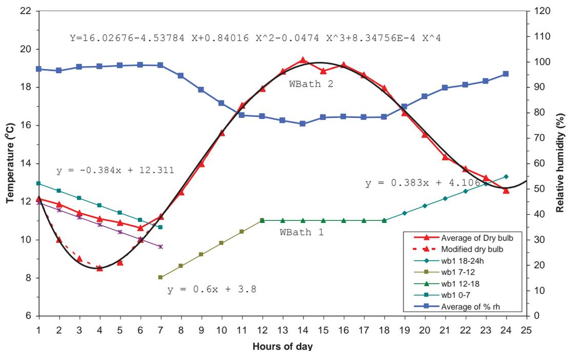
Mean 24-hourly temperature and relative humidity (RH) at Te Puke Research Orchard meteorological site from 1 October–31 December 1996, modified temperature profile used for fitting polynomial and plots of functions used for controlling the set points of waterbath 1 and 2 to achieve diurnal fluctuation of temperature and RH.
