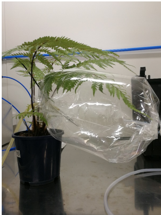
Figure 2-6. Example of a laboratory experimental setup of the dynamic volatile headspace collection system using a PVAS22 unit on D. squarrosa .
