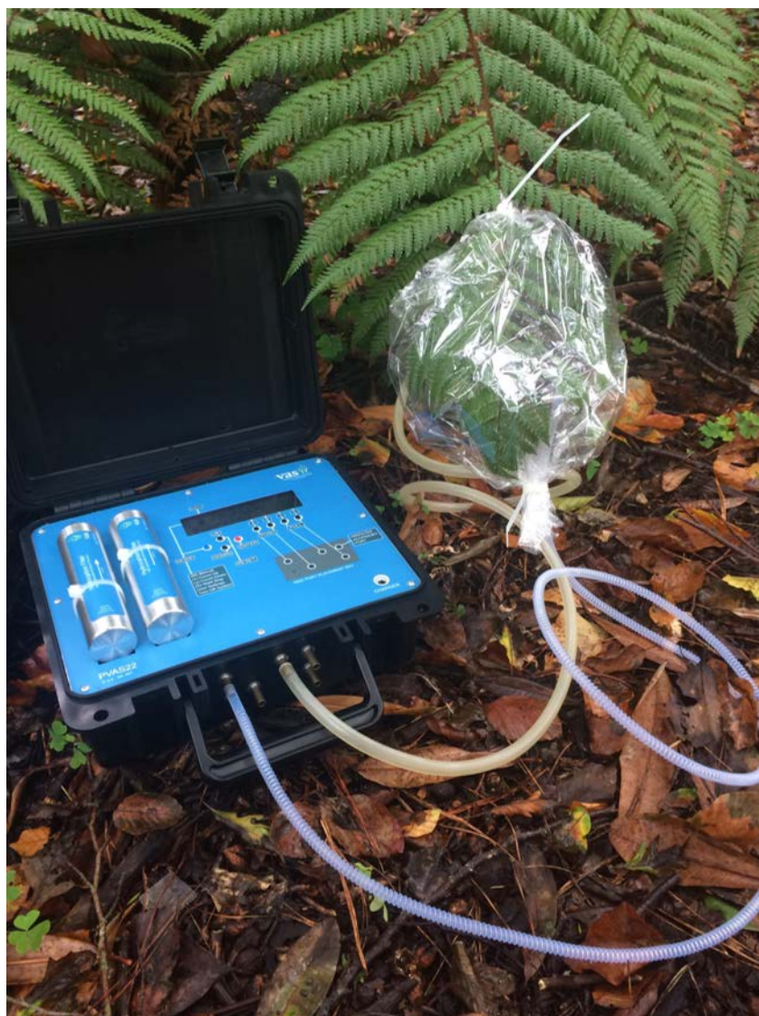
Figure 2-4. Example of a field experimental setup of the dynamic volatile headspace collection system using a PVAS22 unit on Dicksonia squarrosa .
