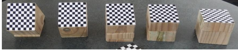
Figure 3.5-Calibration Blocks A45, A30, A20, A10, A0, with Texture T5
