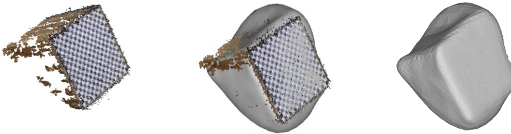
Figure 5.17 – Poisson Meshing of SFM point cloud
