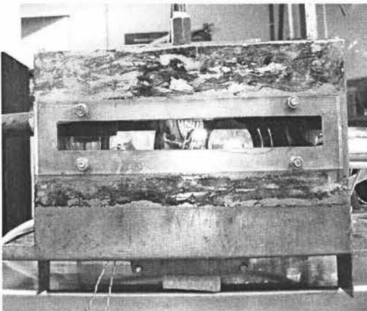
Figure 3-8: Smearing trial set up.
