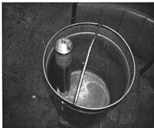
Figure 3-5: Water bath & cylinder to hold the lactose solution.
