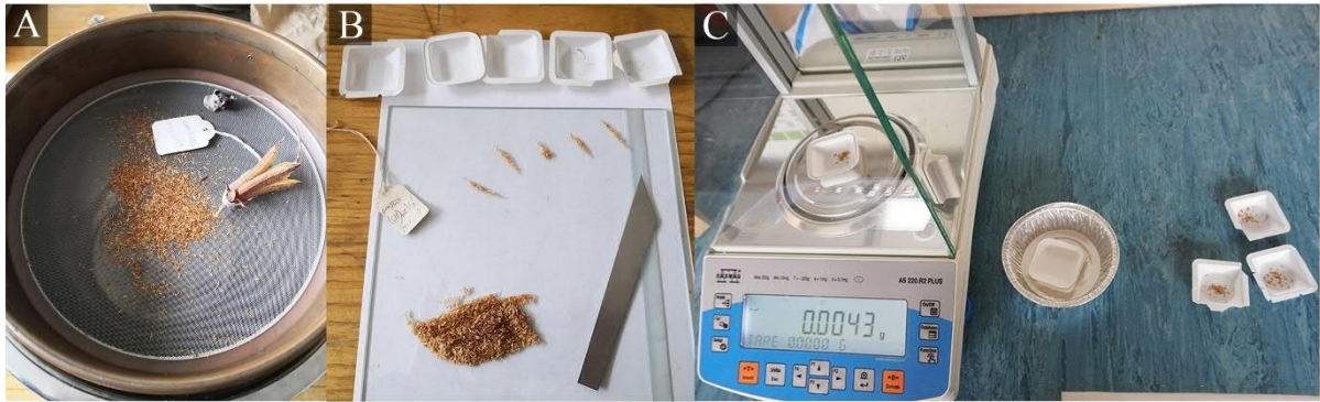
Figure 5.3 Cleaning seed capsules and measuring seed weight. A) cracking seed capsules, removing debris, and filtering seeds with a sieve (355 mic); B) counting 50 seeds for each of five lots; C) weighing each lot of 50 seeds
