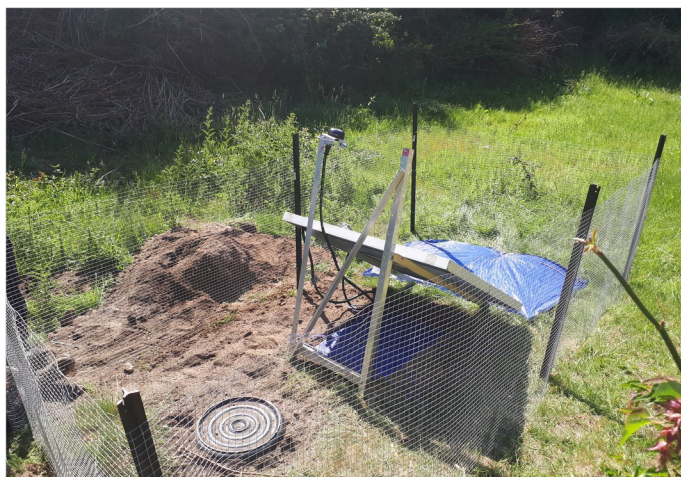
An example seismometer, buried underground
