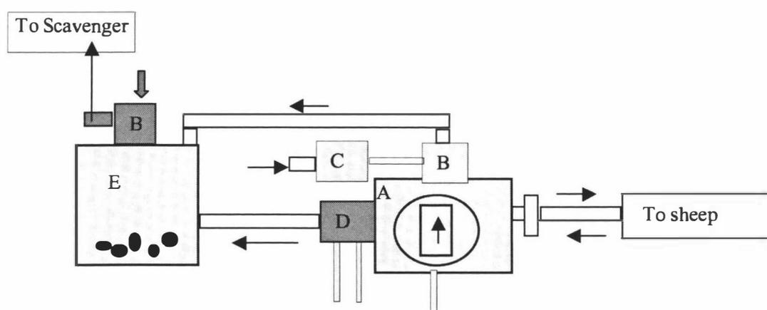
**Figure 4.1. The arrangement of apparatus used for antigen/PBS exposures in conscious sheep. A= two-way valve, B= one-way respiratory valve, C= nebuliser, D= Pneumotachograph, E= Vapour trap,  $\rightarrow$  = flow direction**
