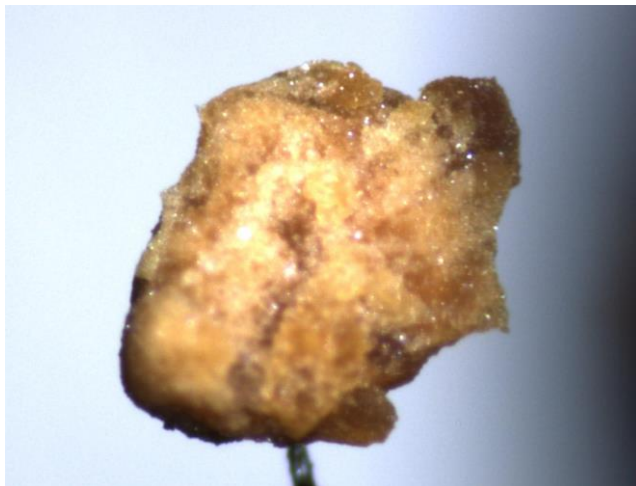
Figure D-1 Picture of a mounted PCN-333 (Fe) sample during a typical PXRD experiment.
