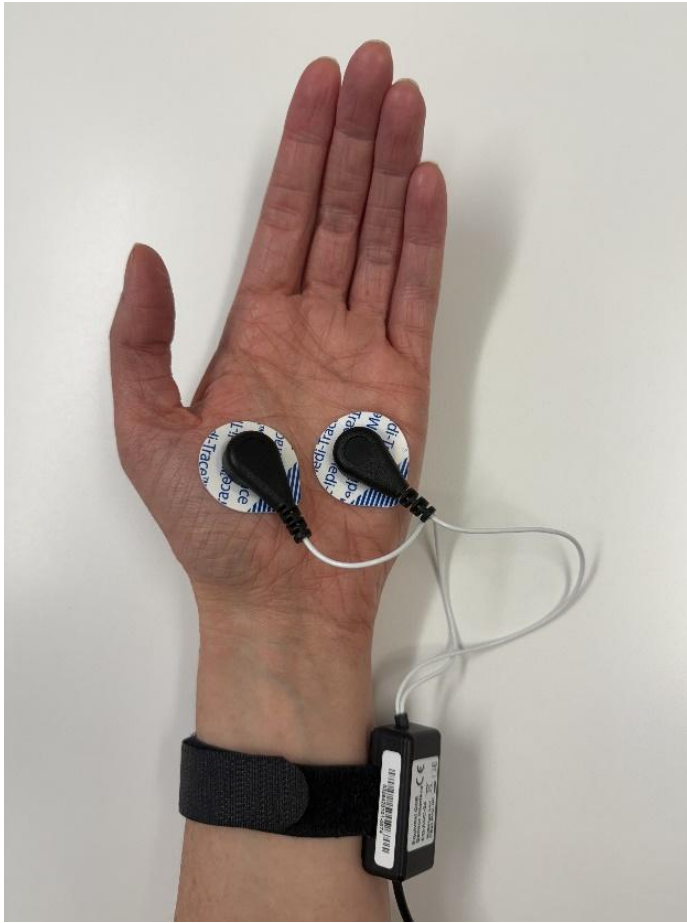
Figure 5. The Equivital galvanic skin response (GSR) sensor with disposable electrodes placed on the palm to measure palmar eccrine sweat gland activity.
