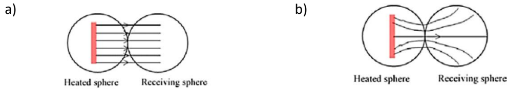
Figure 3-1, Heat flow pathway for high product to medium thermal conductivity ratio (a) and low ratio (b), adapted from Laguerre, Amara, and Flick (2006)
