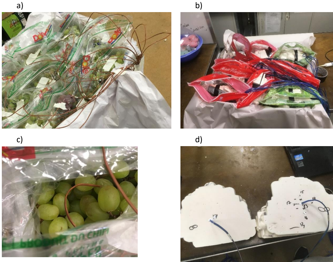
Figure 6-11, Experimental setup for table grape and bulk table grape simulator experimental, a) table grapes, b) bulk table grape simulator, c) thermocouple in table grape berry, and d) thermocouples in fixed positions
