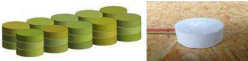
Figure 2-14, The cheese simulator in the Pham, Moureh, and Flick (2018) study
