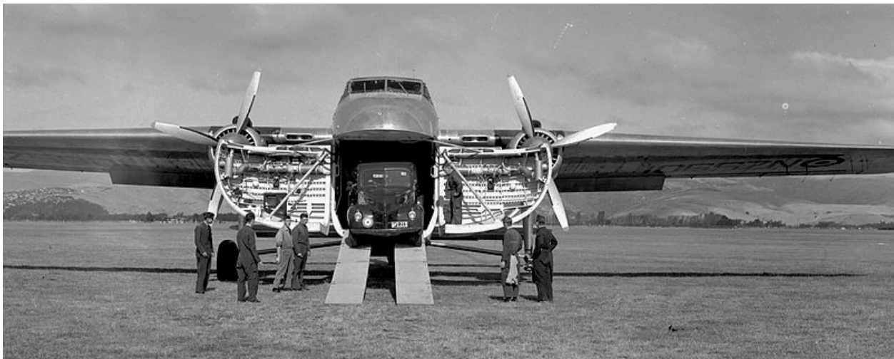
A RNZAF Bristol Freighter showing the distinctive clamshell doors. (Source: AFMNZ, WgG2510-52)
