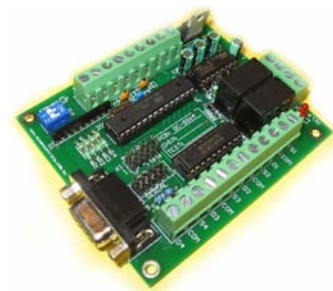
Fig. 2. The Ocean Controls motor controller (KTA – 190) [18]
