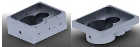
Fig. 10. Original motor mount (left), redesigned motor mount with excess material removed (right)
