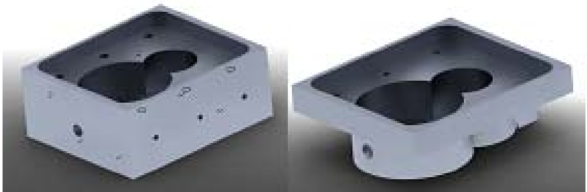
Figure 16: Solidworks Images of redesigned parts to reduce excess weight.
