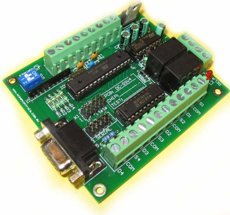
Figure 23: Ocean Control KTA-190 Serial Stepper Motor Controller. ( www.oceancontrols.com.au )
