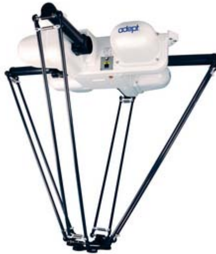
Figure 9: Parallel robot design. ( http://iccrobotics.com/robot_parallel.html )
