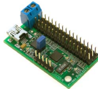
Fig. 5. Pololu USB 16-servo controller board
