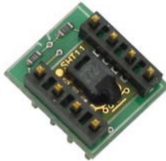
Figure 44: Parallax Sensirion SHT11 Temperature and humidity sensor. ( www.parallax.com )
