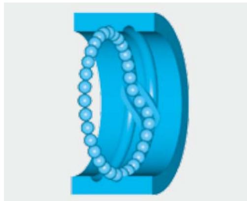
Figure 10: Cut away of how a ball screw operates. Source: Hiwin Data Sheet
