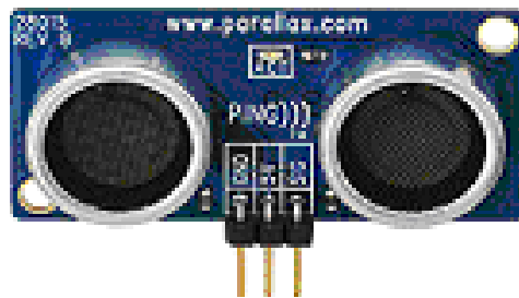
Figure 42: Parallax Ping)))™ ultrasonic proximity sensor. ( www.parallax.com )
