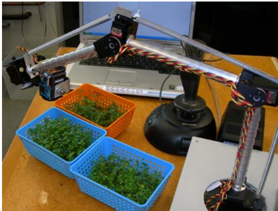
Fig. 14. The completed robotic arm with camera, joystick and plant trays
