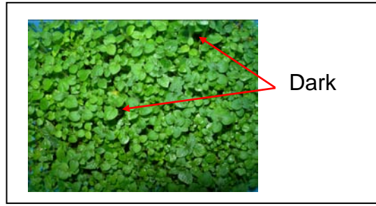
Figure 5. Captured image showing areas of "darkness" caused by overlapping which would lead to false colour readings
