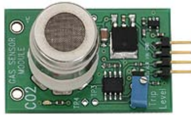
Figure 46: Parallax CO 2 gas sensor module. ( www.parallax.com )
