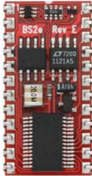
Figure 47: Parallax Basic Stamp 2e Microcontroller. ( www.parallax.com )
