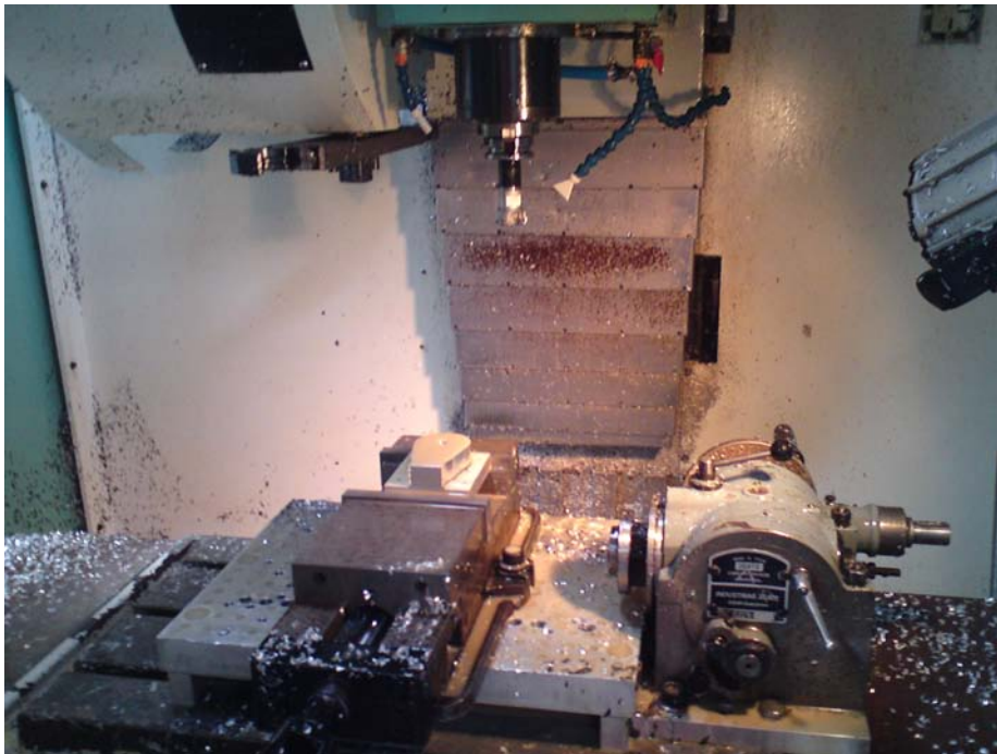
Figure 20: CNC machine in use machining a component out.
