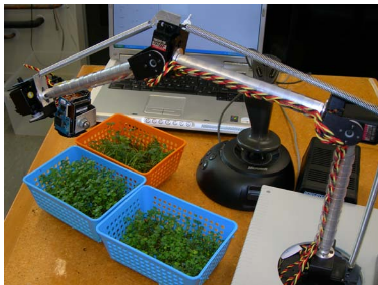
Figure 1: Robotic arm designed as part of Honours project
