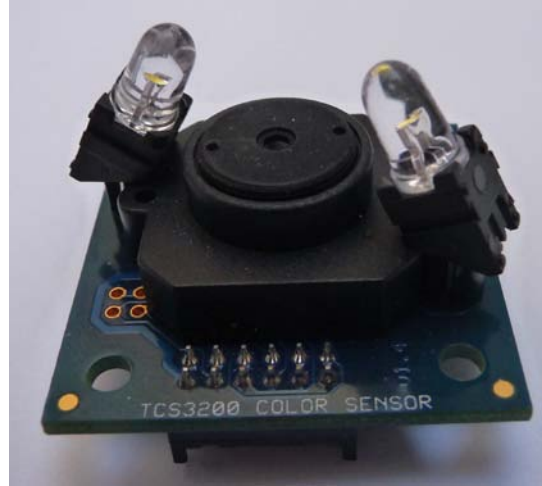
Figure 32: Parallax TCS3200-DB RGB colour sensor.
