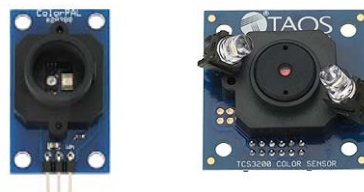
Fig. 5. Parallax ColorPAL (left) and Parallax TSC3200 (right) colour sensors [17]
