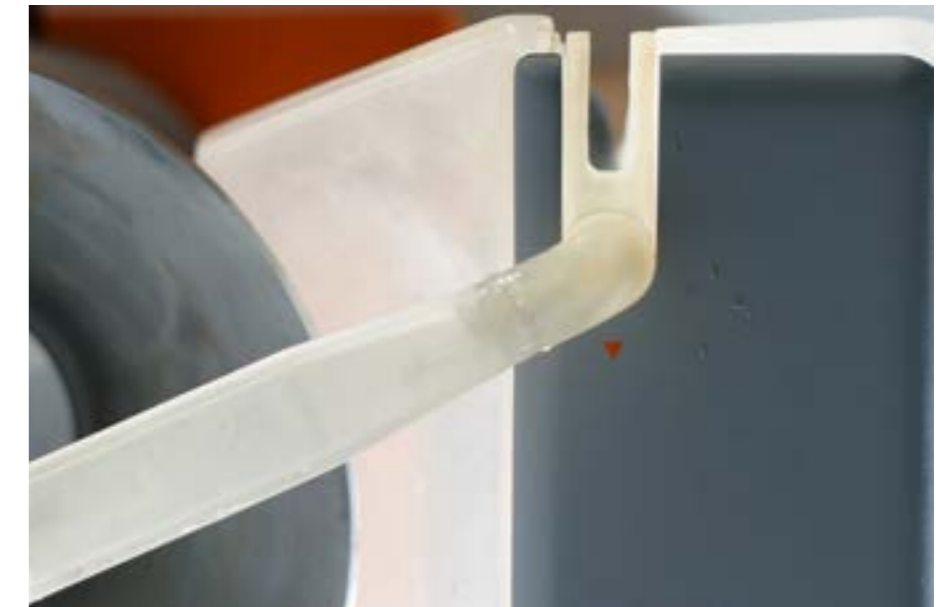
Vinyl cut iconographic stickers were created but were too small and many failed so were not used. This was inspired by the HP Z800. Larger painted or water transfer instructions might work better. Better instructions will have to be developed
