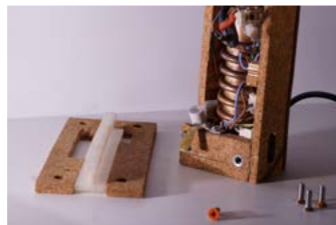
Removable panels from two sides for access to repair and replacement of components. every component could be disassembled
