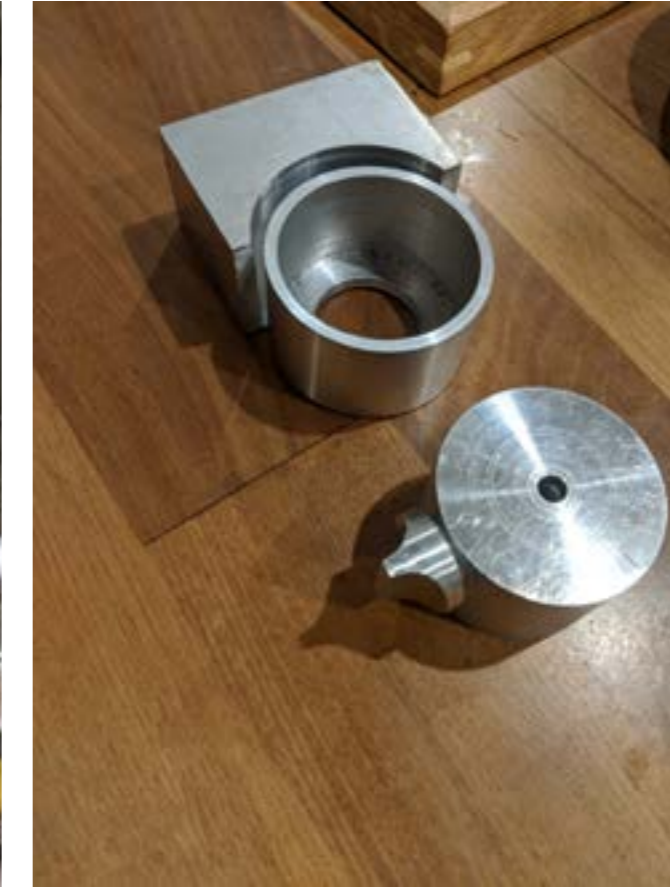
Valve was found to act as heat sink during testing and will have to be hollowed to improve coffee temperatures.
