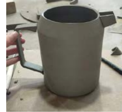
Initial suspended handle design became chunky to support weight and not sag before firing
