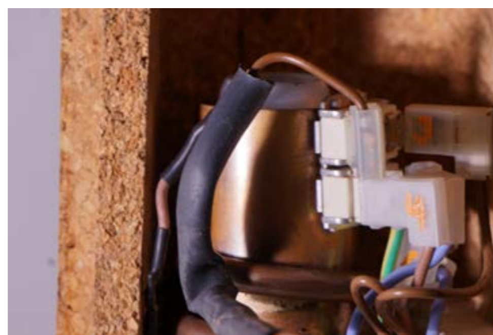
Quick release sliding fittings were used for cables, removing the need for soldering. These had numbers that corresponded to connection points.
