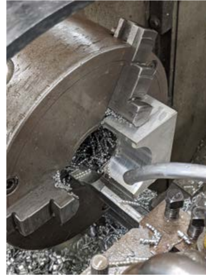
Valve was found to act as heat sink during testing and will have to be hollowed to improve coffee temperatures.
