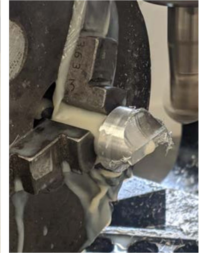
Valve was found to act as heat sink during testing and will have to be hollowed to improve coffee temperatures.
