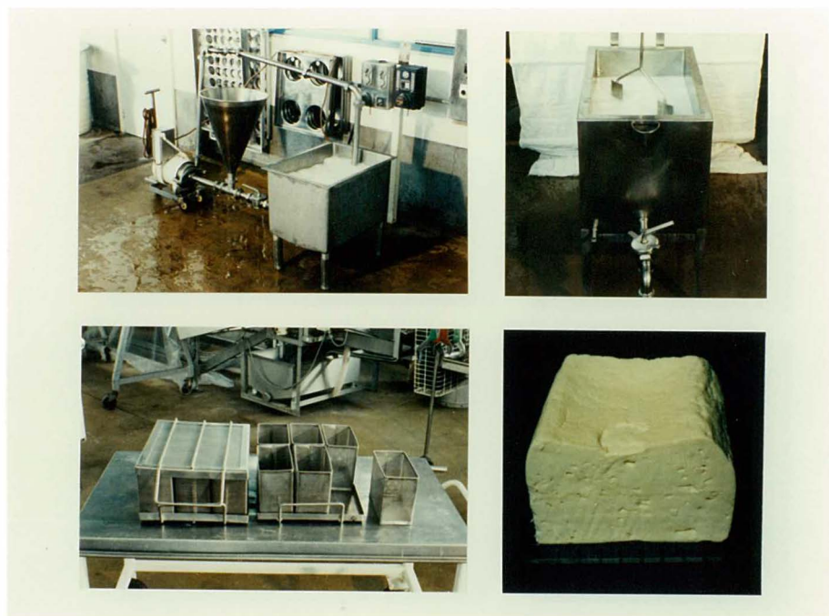
Fig. 6.2 Selected stages in Feta cheese manufacture.
