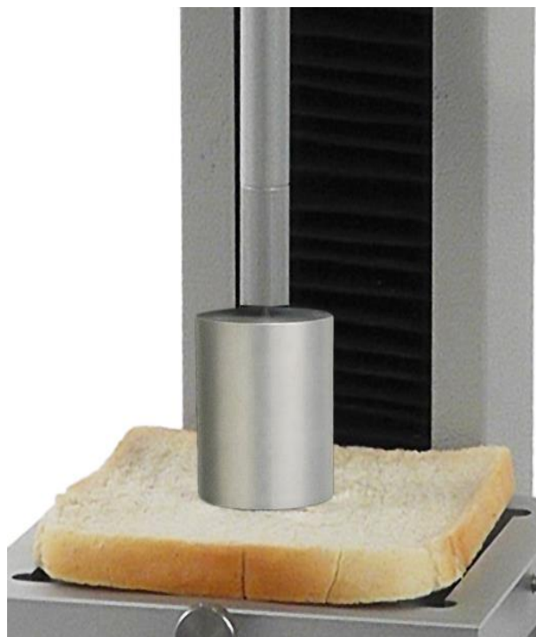
Figure 2.7 Texture analysis of white bread with 36mm cylinder probe attachment
