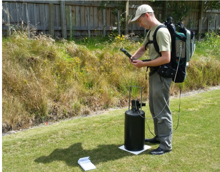
Figure 3.3: ASD FieldSpec© 4 with attached CAPP in operation (white reference standard being collected).
