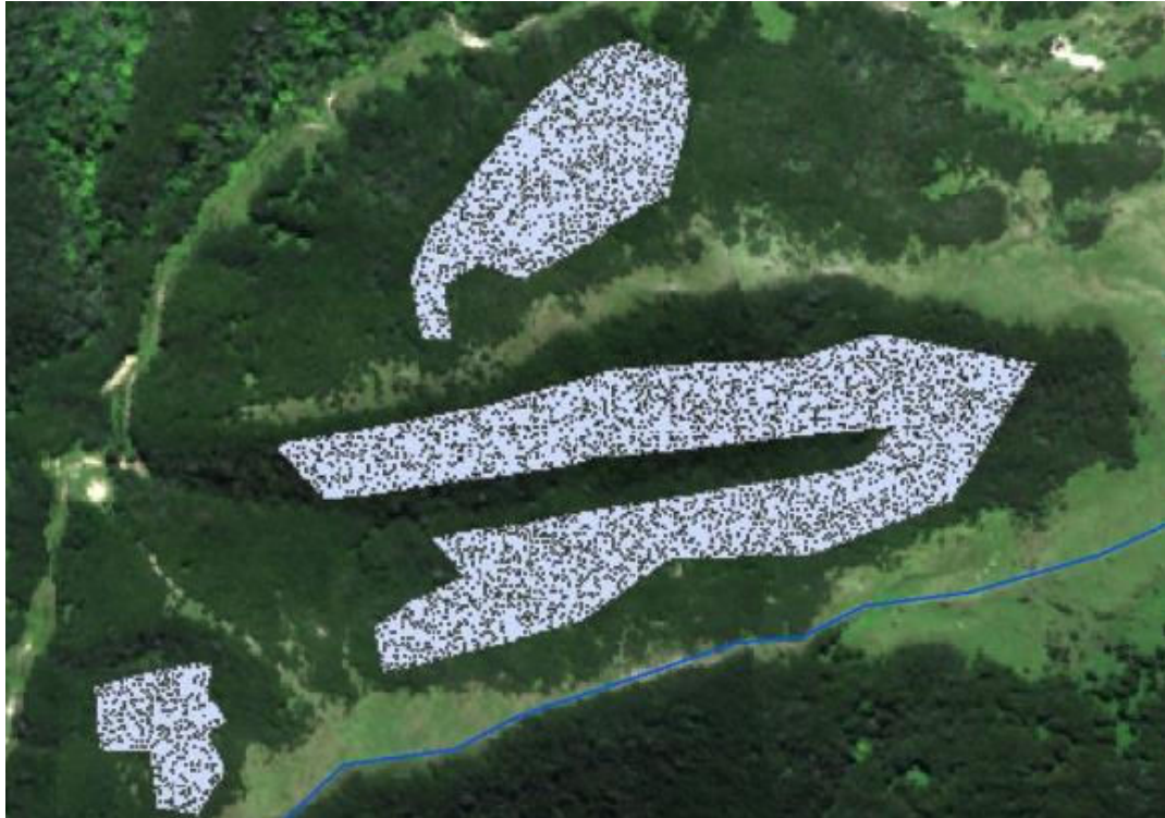
Figure 6.2: ROI polygons (blue) designated for manuka and overlaid on the true colour image. The blue line is a paddock boundary fence location. Missing pixels (dark points) within the ROI are where pixels were randomly removed for training the classification. Each pixel is approximately 0.8 - 1 metre for scale.
