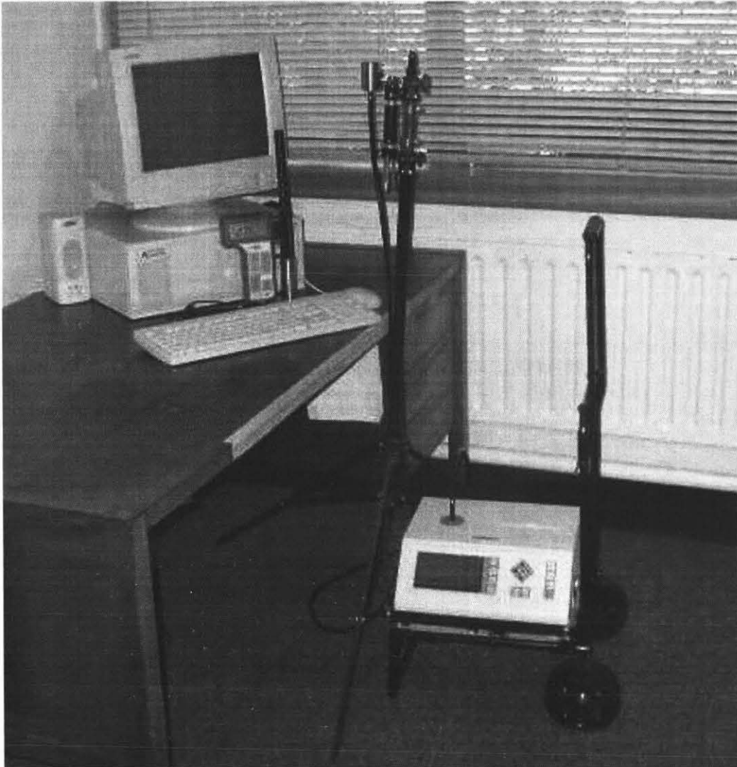
Figure 2. Representation of Metone 3113 particle counter on trolley with isokinetic probe attached to tripod during sampling of particle concentrations in a participant building.
