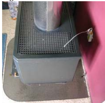
Figure 3.4: Wood burner with a thermocouple attached to the external surface.
