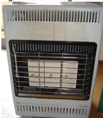
Figure 3.3: Unflued gas heater with a thermocouple located in the middle of each panel.
