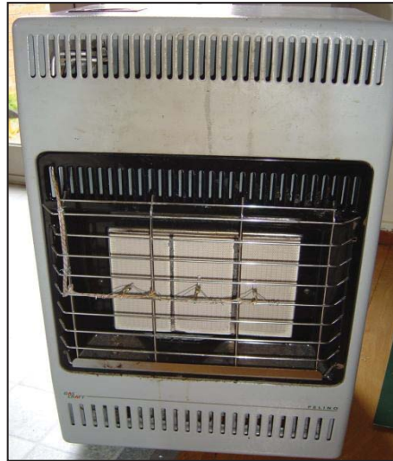
Thermocouple connected to an UGH
