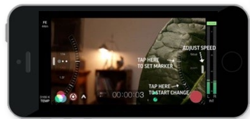
Figure 95: Third-party applications such as Filmic Pro offer a programmable focus dial, often inaccurate enough for complicated camera movements where focal points are changed multiple times.
