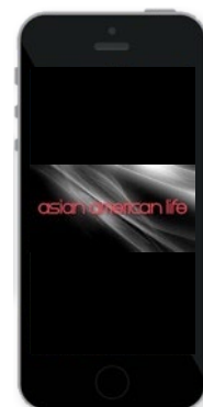
Figure 84: By weird look, Ernabel refers to large letterboxes exhibited when 16:9 footage is watched at a 9:16 aspect ratio screen without a blow-up.
