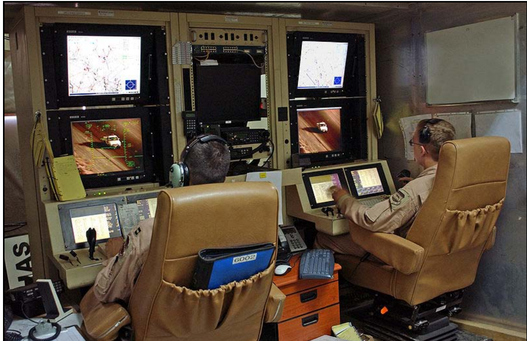
Fig 6. The interior of a Predator Ground Control Station (GCS)
