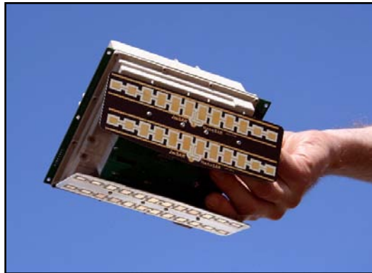
Figure 8. NanoSAR weighs in at two pounds
