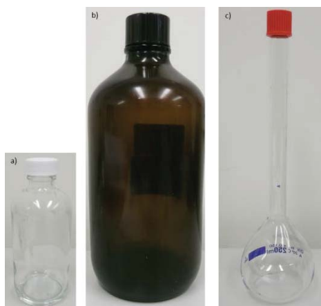
Figure 3.4: Photographs of the different sample bottles tested: a) 125 mL sample bottle, b) 1000 mL sample bottle, and c) 273 mL sample bottle.
