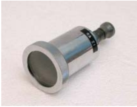
Figure 2.6: Image of a Lucas Cell used for measuring radon. The large circular base of the cell comprises a glass window which will be captured by a connected photomultiplier. Image retrieved from (Lenzen & Neugebauer, 1996).
