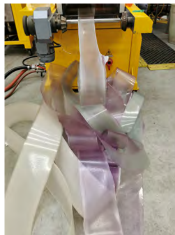
Fig. 6, 7. Documentation of lab work with Beatrix Theobald at Scion, a crown research institute in Rotorua. The film extruder machine at Scion is used to melt and blend pellets of bacterial and plant-based polymers. Pigments are added at intervals, creating a spectrum of colour as the mix moves through the machine and heated rollers press and stretch molten polymers into a thin film.
