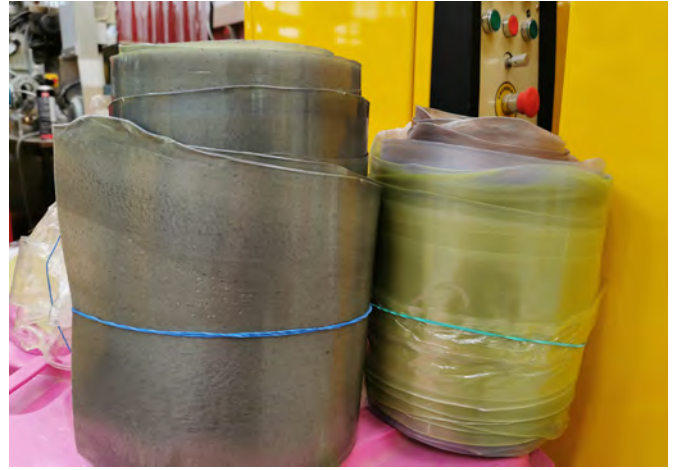
Fig. 18,19. DIY pigments ground from greywacke quarry rock fall and extruded into rolls of bacterial polyester at Scion. The film extruder machine at Scion is used to melt and blend pellets of bacterial and plant-based polymers. Pigments are added at intervals, creating a spectrum of colour as the mix moves through the machine and heated rollers press and stretch molten polymers into a thin film.
