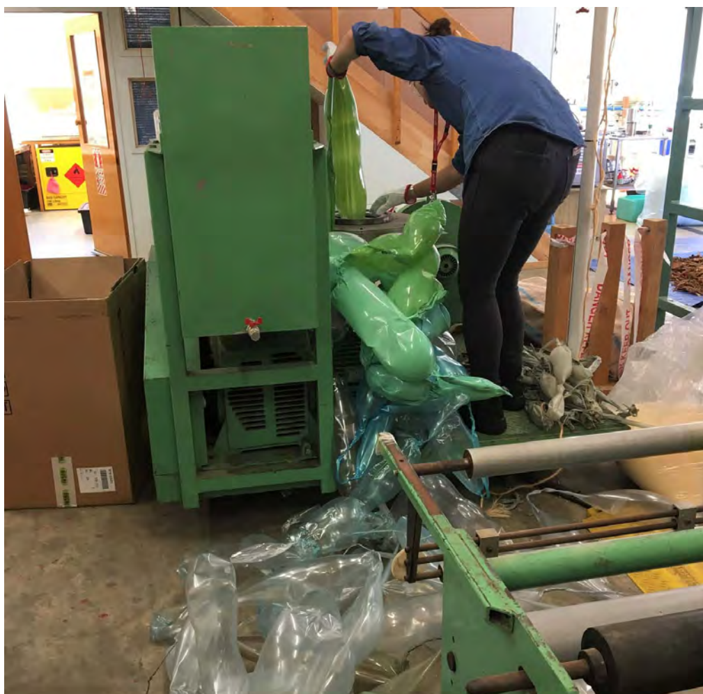
Fig. 33, 34. Documentation of lab work with Beatrix Theobald at Scion, a crown research institute in Rotorua. The extruder machines at Scion are used to melt and blend pellets of bacterial and plant-based polymers.
