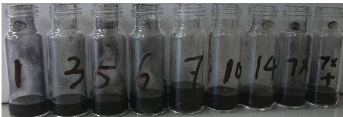
Figure 4-4. Effervescence tests for carbonate-C in biochars. Numbers are the samples numbers in Table 4-1. Sample “N o 7x” is sample N o 7 after acid treatment; “N o 7x+” is “N o 7x” plus 5mg of dry CaCO 3 .
